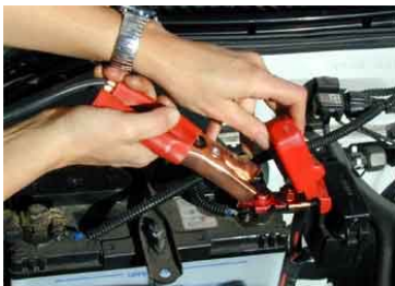
Positive to Battery Terminal
