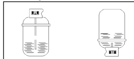
Fig. 13: Virgin refrigerant cylinder tank types
