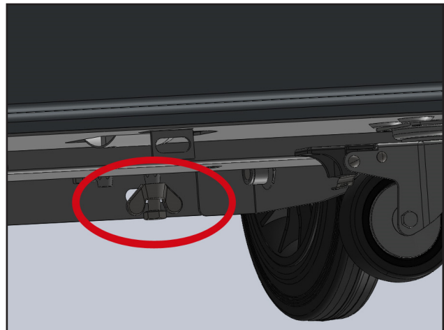
Fig. 12: Removing load cell retention bolt
