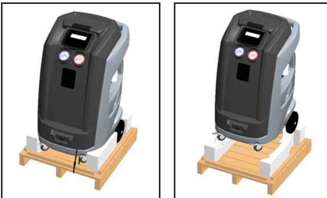
Fig. 10: Tilting unit backwards
