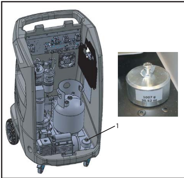
Fig. 33: Reference weight location
