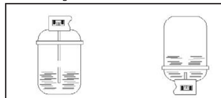
Fig. 13: Virgin refrigerant cylinder tank types
